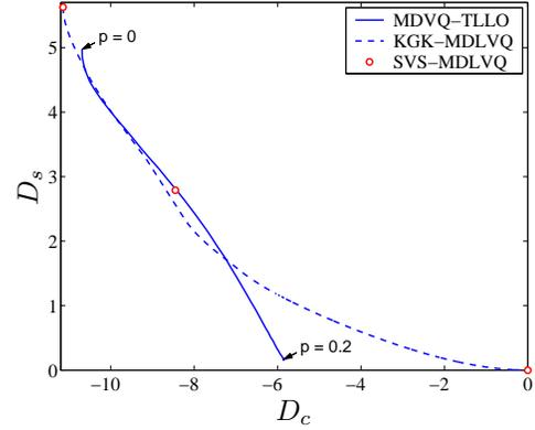
Fig. 3. Performance comparison of normalized central and side distortions in dB. A few channel optimized operating points of MDVQ-TLLO are highlighted.
