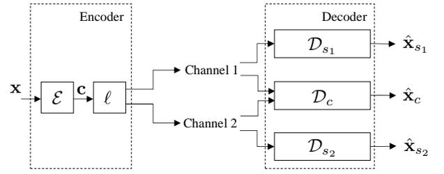
Fig. 1. A block diagram of a multiple-description quantizer.
